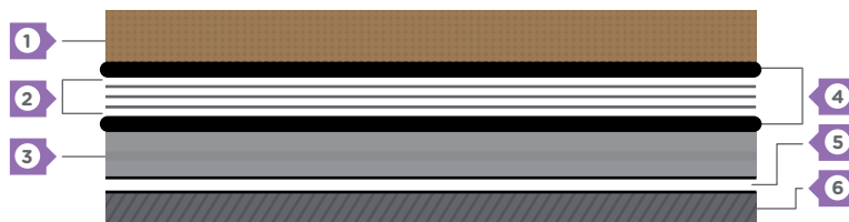
Cross-section diagram: Four-ply built-up roofing
