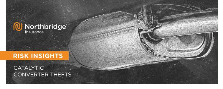
Many Canadian cities are reporting an increase of catalytic converter thefts. A Catalytic Converter is a specific and valuable part of a vehicle's exhaust system. They're made from layers of precious metals designed to reduce many of the toxic emissions created by a vehicle's engine. This car exhaust component can be made up of precious metals such as platinum, palladium, and rhodium which make this part very appealing to steal and resell for high value.
